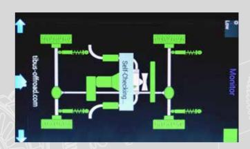
This high-resolution display shows a graphical layout of your vehicle with easily recognizable symbols and figures, allowing you to control the temperatures of your vehicle's components at up to 18 measuring points.
