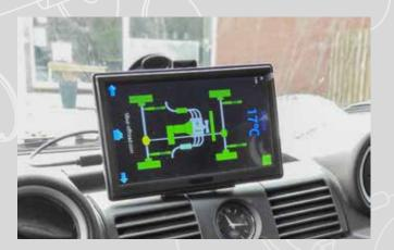
With a simple tap on the display, you're able to recall the temperature at the measuring point at anytime. The maximum temperature reached is stored in the file system and can be retrieved. Problems can be detected and remedied in time far before you hit the outback and get would otherwise get stuck in the middle of nowhere.
