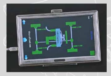
With the TIBUS temperature monitor "TMS18" you will never lose sight of all the important temperature data of your vehicle. You can identify deviations at first glance on a 5" touch-screen monitor.
